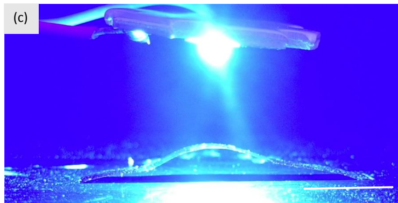
Figure 4- 5. (a) A curved 1 mil Kapton film after annealing in an oven for 24 hours at 120°C. (b) Deposition of the azobenzene MeOABHx polymer on top of the passive Kapton film causes the film to contract and form a straight shape. (c) When activated by blue light (455 nm), the film rises by 2.33 mm. Solid white bars represent a scale bar of 10 mm in length.
