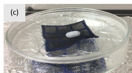
(c) When the PLA Fabric encapsulation is placed into 70°C water it unfolds and releases the stir bar
